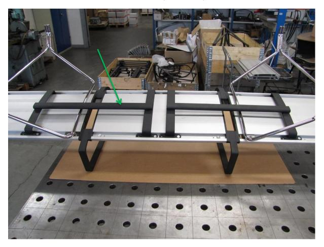
The reinforcement brackets are screwed on to the profiles with predrilled holes (X) (M6x16)
