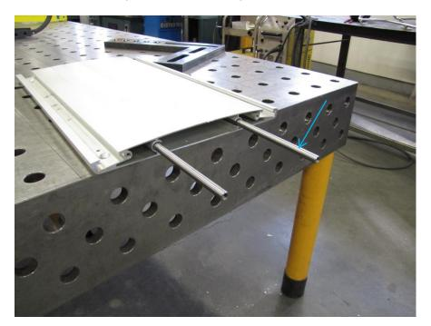
The threaded rod is pushed into the seat profile and locks with screw from each side (M8).
