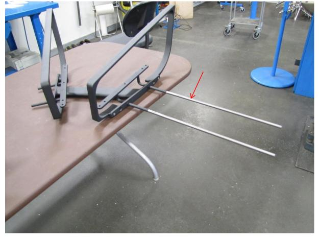
The **Threaded rod for end** is screwed on to the table stand.
